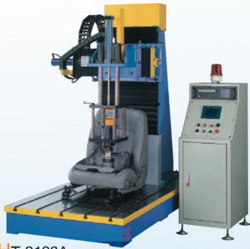
HT-2123A 座椅乘降耐久試驗機 Getting In / Out Durability of Seat Cushion Tester
